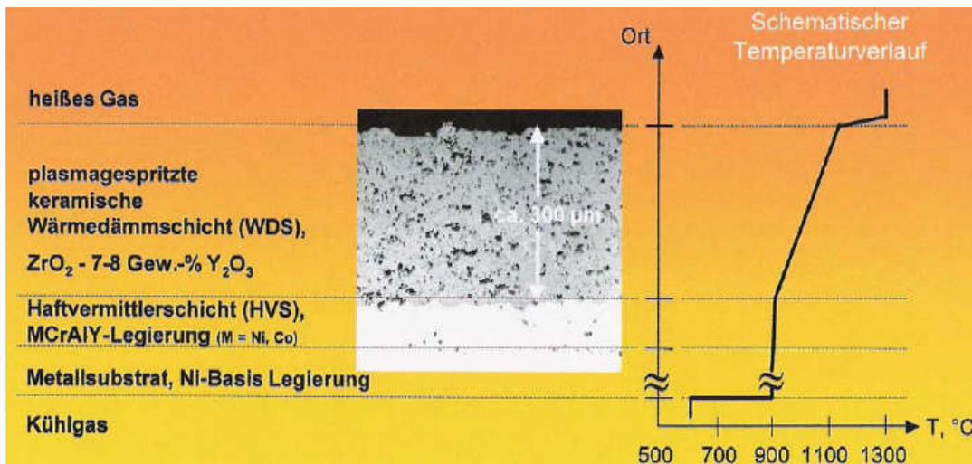
Figure 2: Schematic Temperature Profile [14]
