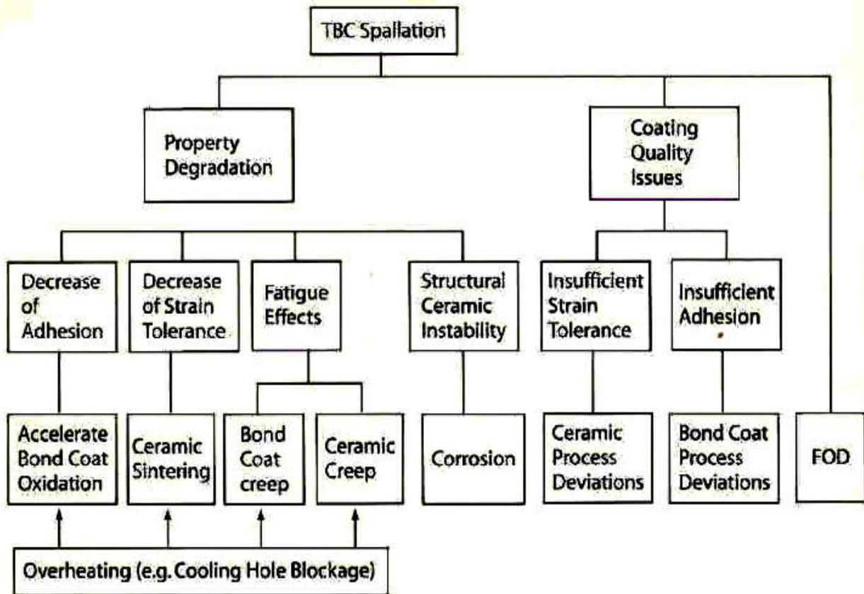
Figure 3: TBC failure overview [15]
