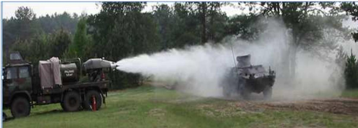
Figure 2. High decontamination unit WUS-3 in marching position with a protective tarp removed and mounted cab
