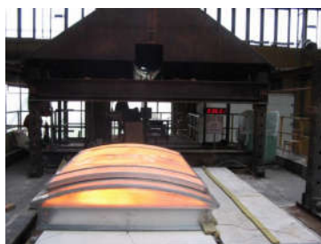
Picture No. 3, air shaft VARASS with SEP ZOKT window after 5 minutes of testing resistance against heat according to the CSN EN 12101-2 in a testing room.
