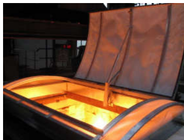
Picture No. 4, air shaft VARASS with SEP ZOKT window after the activation during testing the resistance against heat according to the CSN EN 12101-2 in a testing room.
