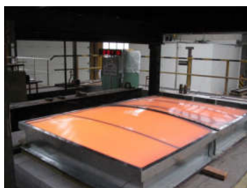
Picture No. 1, SEP ZOKT flap after starting the resistance against heat according to the CSN EN 12101-2 in a testing room.
