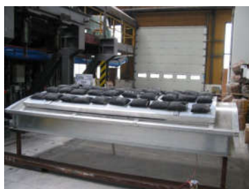
Picture No. 2, air shaft VARASS with SEP ZOKT window during a test of the resistance against snow loading according to the CSN EN 12101-2 in a testing room.
