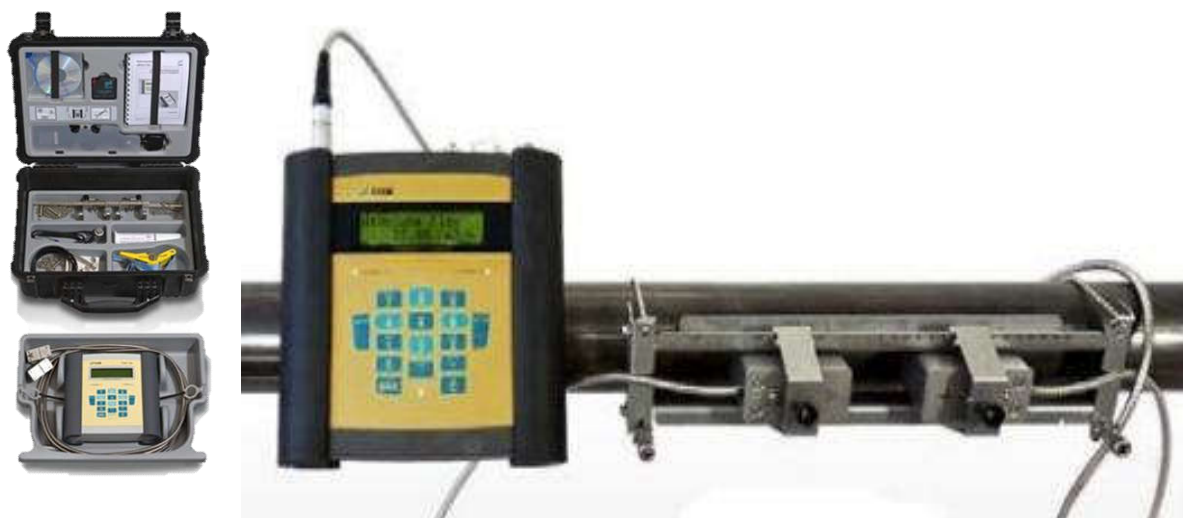
Figure 3 Flow monitor FLEXIM G608 10 and flowmeter set 11
