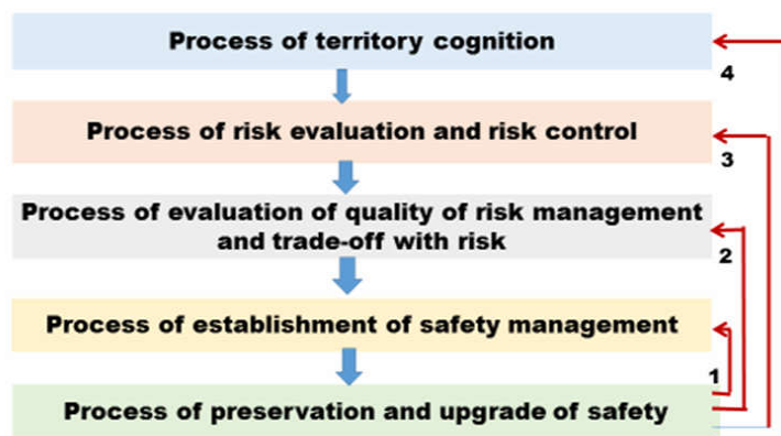
Fig. 8 - Structure of super process for risk management and trade-off with risk for profit of safe territory and safe public assets. The numbers denote the feedbacks that need to be realised if problems occur. From the economy reasons the firstly the feedback 1 is applied, and only if it fails the feedback 2 etc.
