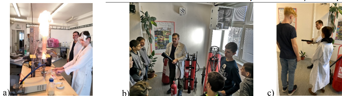
Fig. 6 The burning of dispersed powder in the Hartmann tube (a) and the presentation of different types of extinguishing agents (b, c)
